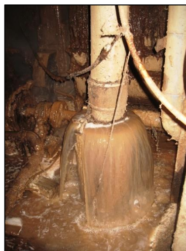
Separator seal tank overflowing indicating flooded vacuum foil element
