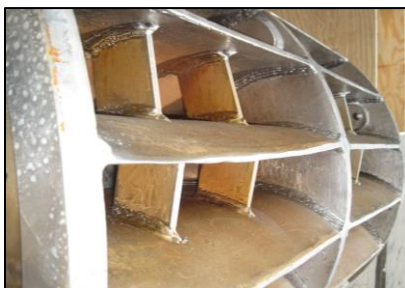
Two fabricated stainless steel rotors for the same pump model – right is OEM. Left side tested at 65% of new performance.
