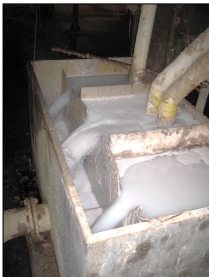
Typical seal tank with weirs – can easily be modified with addition of level transmitters
